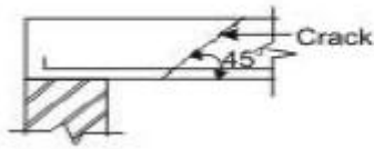
Figure 1.10 (a) Web shear progress along dotted lines
